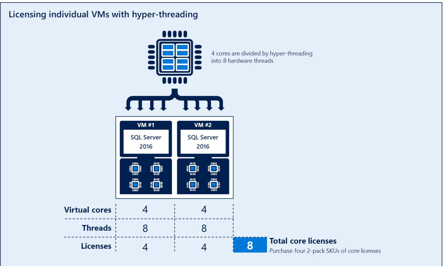
A four core processor with hyper-threading supports two VMs with four virtual cores each.
