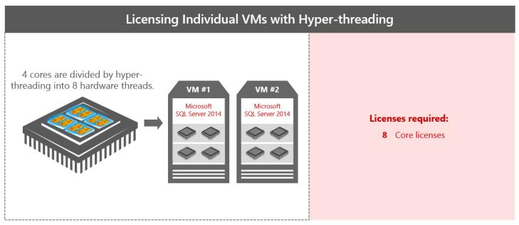
In this figure, a four core processor with hyper-threading supports two VMs with four virtual cores each.
