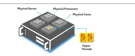
Hardware thread: A hardware thread is either a physical core or a hyper-thread in a physical processor.
