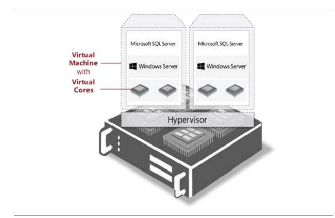
Figure 4: Virtual Machine (VM) using virtual cores
